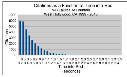
This is the typical distribution of red light running events seen for the straight through movement when the yellow interval is set at or near the minimum time based on the posted speed limit. When the yellow interval is increased, violations occurring during the corresponding time period are eliminated.
